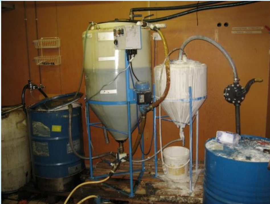
Biodiesel production from used vegetable oil On a farm in Parikkala Finland
